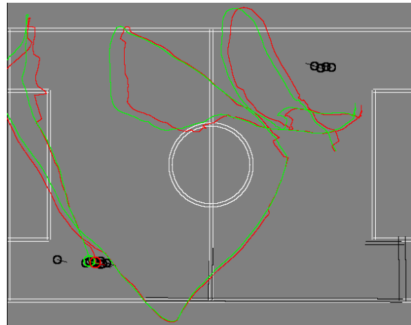
Figure 1: Comparison of actual (green) and estimated (red) trajectories as well as current projection and position hypotheses (black)
